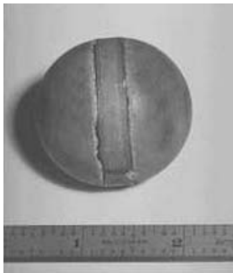
Figure 3. Plutonium 238 oxide sphere.
